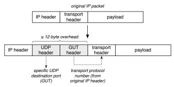
(a) Generic UDP Tunneling (GUT) [81], allowing encapsulation of an arbitrary native transport protocol.
