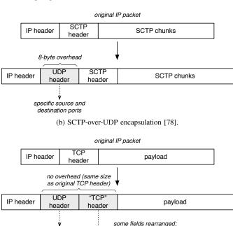
Fig. 2. Examples of transport encapsulation methods based on UDP.
