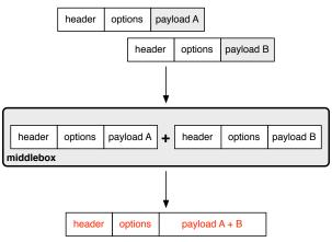
(d) Coalescing of small TCP segments into a single, larger segment: parts of the header are rewritten, and options in the coalesced segment may change.
