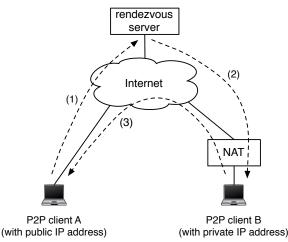
(b) Connection reversal: (1) A sends a connection request to a rendezvous server to which B is connected; (2) the server relays the request to B; (3) B connects to A. Use of a server and higher connection-setup latency are potential performance issues. (Adapted from [18].)
