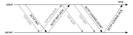
Fig. 5. "Happy eyeballs" technique for the discovery of SCTP support, with SCTP being the preferred choice. The first handshake of the SCTP association succeeds shortly after the TCP connection does, so the latter is aborted.
