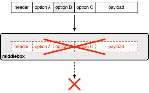
(b) Blocking of TCP segments due to unrecognised TCP options: the segment is dropped.
