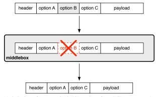
(a) Stripping of unrecognised TCP options from TCP segments: the segment is forwarded but the unknown option is removed.
