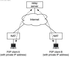
(d) Relaying: the relay server relays data between the connections from A and B. Use of a relay server can be a performance bottleneck. (Adapted from [18].)
